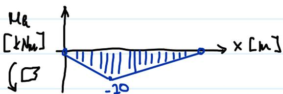
$$\text{I: } \sigma_{\text{meg}} = \frac{M_k(x_{\text{knt}}^{\text{I}})}{I_y} \cdot \frac{b_1}{2}$$
