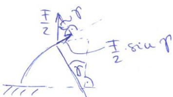
$$M_{\text{a}}(\gamma) = M_B - \frac{F}{2} \cdot \sin \gamma \cdot R \rightarrow \frac{\partial M_{\text{a}}(\gamma)}{\partial M_B} = 1$$
