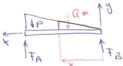
$$M_n(x) = -F_B \cdot x + \underbrace{\left(\frac{p}{3L} x\right)}_{\text{erd}} \cdot \underbrace{\frac{x}{2}}_{\text{erd}} \cdot \underbrace{\frac{x}{3}}_{\text{erd}} = -\frac{1}{2} L p x + \frac{p x^3}{18L}$$
