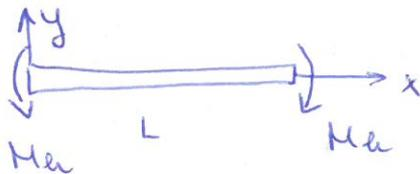
$$\underline{\underline{\sigma}} = \begin{bmatrix} \sigma_x & 0 & 0 \\ 0 & 0 & 0 \\ 0 & 0 & 0 \end{bmatrix}$$
