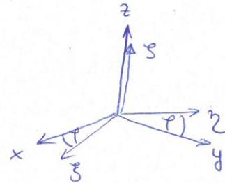
$$\underline{\underline{I}}_S = \underline{\underline{\Theta}}_S \cdot \underline{\underline{\omega}} = (\underline{\underline{\Theta}}_1, \underline{\underline{\Theta}}_2, \underline{\underline{\Theta}}_3) \cdot \begin{bmatrix} -\omega \cos \varphi \\ -\omega \sin \varphi \\ 0 \end{bmatrix} = \begin{bmatrix} -0,346 \\ -0,1 \\ 0 \end{bmatrix} \text{ kgm}^2$$
