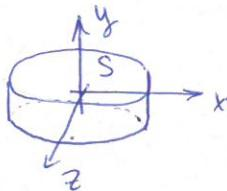
$$\underline{\Omega}_S = \begin{bmatrix} \Omega_{Sx} & 0 & 0 \\ 0 & \Omega_{Sy} & 0 \\ 0 & 0 & \Omega_{Sz} \end{bmatrix}$$
