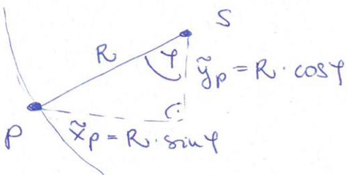
$$1.) \quad \underline{v}_p = \frac{d \underline{r}_p(\varphi(t))}{dt} = \frac{d \underline{r}_p}{d\varphi} \cdot \frac{d\varphi}{dt} = \dot{\underline{r}}_p(t) = R \begin{bmatrix} \dot{\varphi} - \cos\varphi \cdot \dot{\varphi} \\ \sin\varphi \cdot \dot{\varphi} \end{bmatrix} = R \dot{\varphi} \begin{bmatrix} 1 - \cos\varphi \\ \sin\varphi \end{bmatrix}$$
