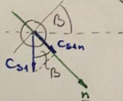
$$c_{s1n} = c_{s1} \cos \beta = \underline{\underline{0,75}} \frac{\text{m}}{\text{s}}$$
