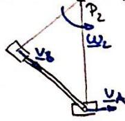
$$v_B = v_A \cos \varphi = v_A \frac{a}{\sqrt{a^2 + b^2}} = 2 \frac{\text{m}}{\text{s}}$$
