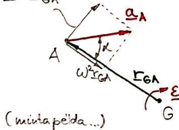
$$\underline{\underline{\alpha}}_A = \underline{\underline{\alpha}}_G + \underline{\underline{\epsilon}} \times \underline{\underline{r}}_{GA} - \omega^2 \underline{\underline{r}}_{GA}$$
