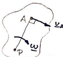
$$v_A = \omega |r_{PA}| \text{ azaz } v_s = \omega r$$
