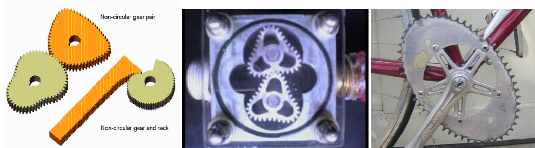
Fig.2. Non-circular gears, non-circular chain-ring and non-linear rack
