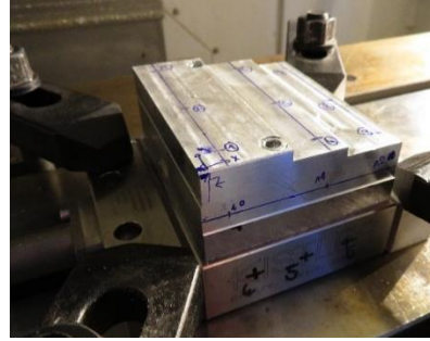
Fig. 1. Test setup. Marked points on the workpiece for modal analysis.
