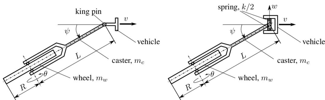
Figure 1: Left panel: the *rigid model* of the towed wheel with two degrees of freedom ( $\psi, \theta$ ); right panel: the *elastic model* of the towed wheel with three degrees of freedom ( $\psi, \theta, w$ ). The third degree of freedom is necessary to model the phenomenon of shimmy
