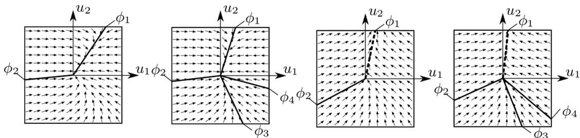
Figure 2: The four generic scenarios of the limit directions in the plane of the slipping velocities  $u_1$  and  $u_2$
