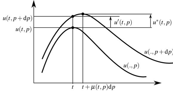
**Fig. 2** Difference between the direct and the generalised parametric sensitivity. In the case of generalised sensitivity, the change of the trajectory is measured by shifting the time variable. The amount of this shift is described by the time dilation function  $\mu(t, p)$ . The figure demonstrates that by an appropriate choice of  $\mu$ , the generalised sensitivity  $u^*$  can measure the effect of the parameter better than the direct sensitivity  $u'$ .
