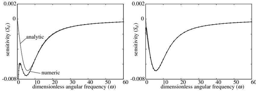
**Fig. 6** Computation of the sensitivities at  $m = 30$ . Left panel: *inappropriately* chosen parameters ( $\alpha = 1$ ,  $\beta = 10$ ,  $n_{div} = 8$ ,  $n_{per} = 5$ ), which cause significant error for small values of  $\omega$  (low frequencies). Right panel: *appropriately* chosen parameters ( $\alpha = 0.1$ ,  $\beta = 100$ ,  $n_{div} = 20$ ,  $n_{per} = 50$ ).
