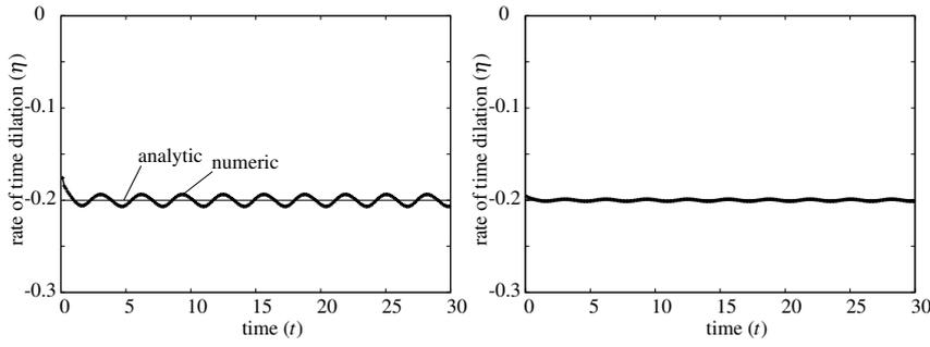
**Fig. 5** Rate of time dilation  $\eta^i$ , by using the parameters  $m = 30$ ,  $\alpha = 1$ ,  $n_{div} = 50$ ,  $n_{per} = 8$ ,  $\omega = 5$ . Left panel: for  $\beta = 3$ , the numerical oscillation is still large, but it remains around the analytical value  $-1/\omega$ . Right panel: for  $\beta = 20$ , the amplitude of the oscillation is small around the analytical value.
