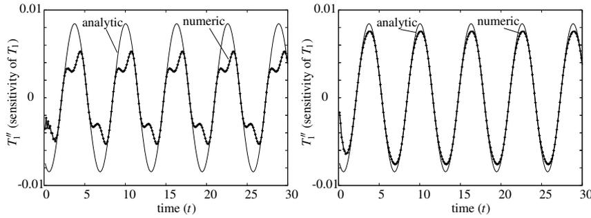
**Fig. 4** Coordinate  $v_1^i$  of the sensitivity of the trajectory, by using the parameters  $m = 30$ ,  $\alpha = 1$ ,  $n_{div} = 50$ ,  $n_{per} = 8$ ,  $\omega = 5$ . Left panel: for small value of  $\beta = 3$ , there is a significant error in the sensitivity. Right panel: by increasing the parameter to  $\beta = 20$ , we get a better approximation.
