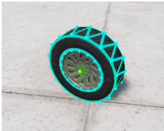
Figure 1: An image of the software tyre model is available in the BeamNG.drive documentation.
