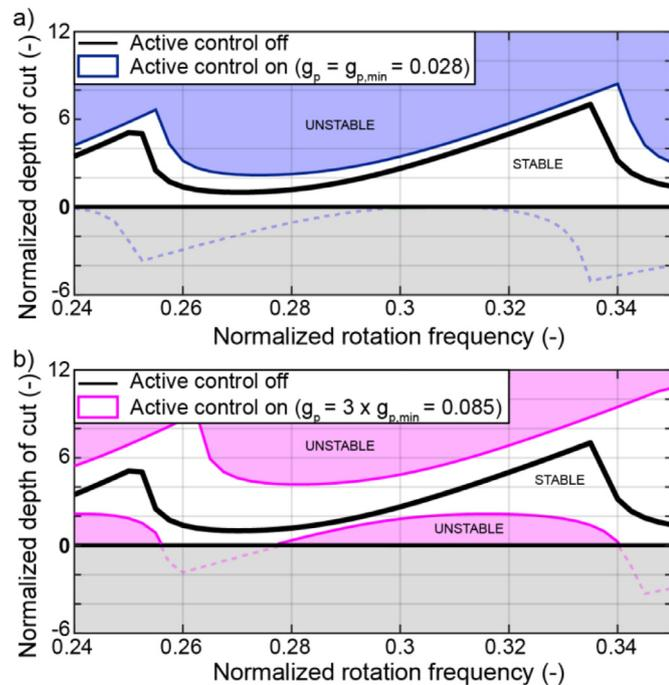
Fig. 3. Effect of the control law over dimensionless stability lobes ( $\xi = 1.4\%$ ;  $n = 4$ ) with an ideal actuator and constant optimum gain. (a)  $g_p = g_{pmin} = 0.028$ ; (b)  $g_p = 3g_{pmin} = 0.085$ .
