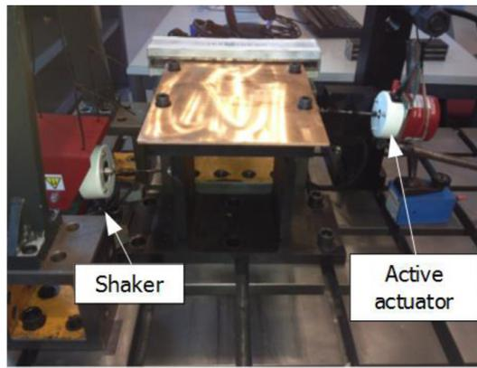
Fig. 6. Hardware-in-the-loop system with the active control loop [28].
