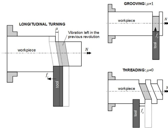
Fig. 2. Scheme of different turning operations.
