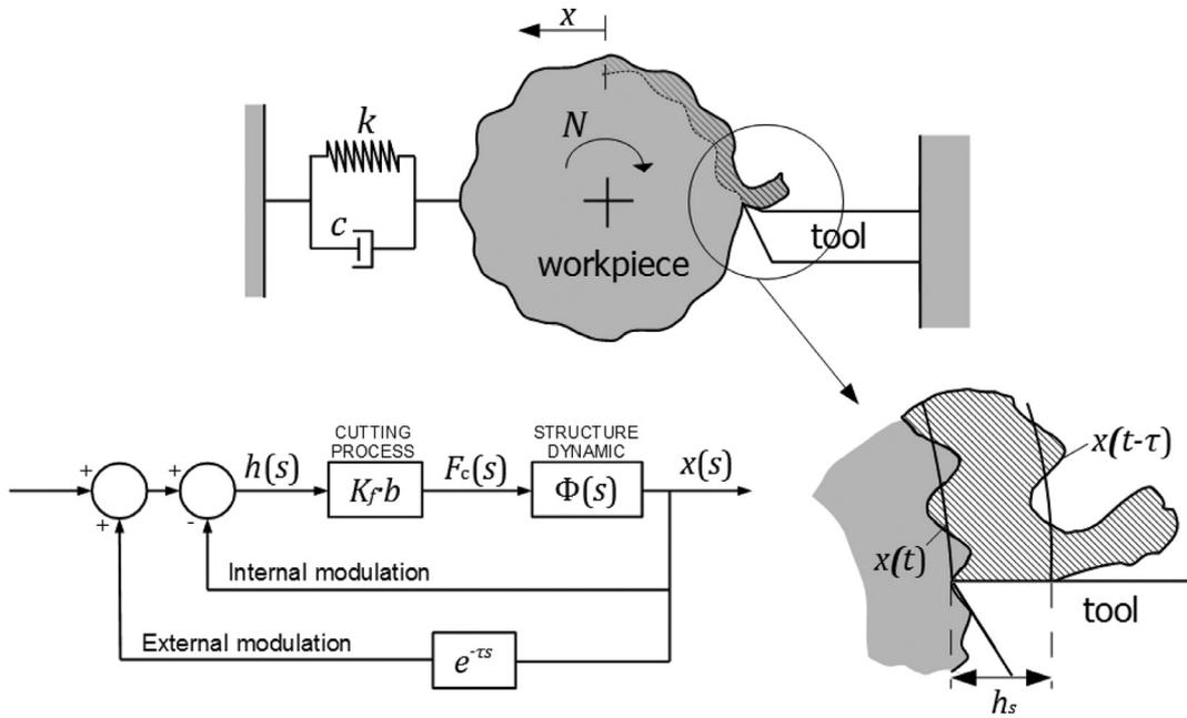
Fig. 1. Regenerative chatter vibrations in orthogonal cutting process [25].
