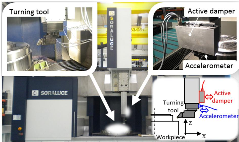
Fig. 9. SORALUCE vertical turning center.
