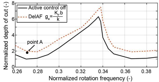
Fig. 7. Hardware-in-the-loop results with and without delayed acceleration feedback control law over fourth stability lobe ( $n = 4$ ).
