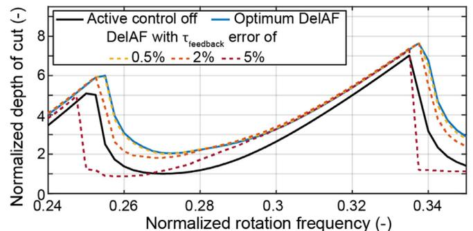
Fig. 5. Delay error sensitivity analysis with DelAF control law ( $g_a = 2\xi\delta_{lim,off}(1 + \xi)$ ,  $n = 4$ ).
