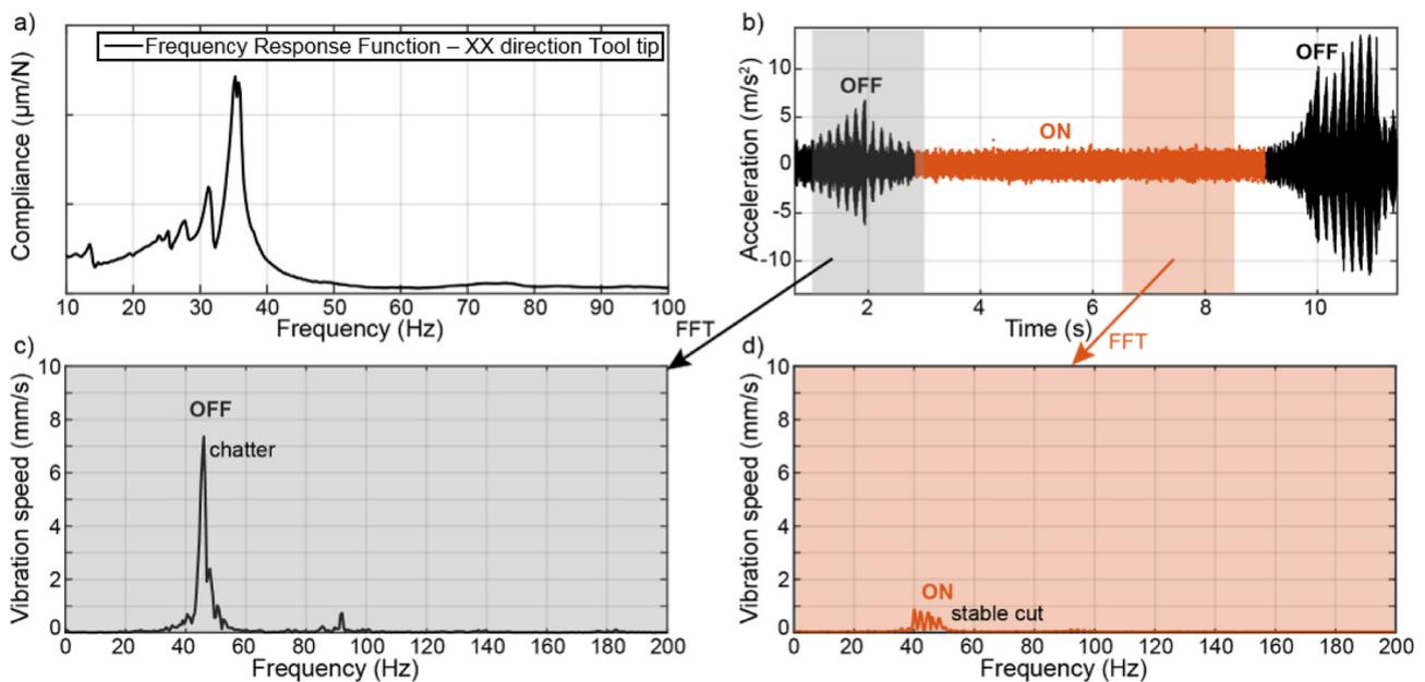
Fig. 10. (a) Dynamical response of the machine structure, (b) effect of the delayed acceleration feedback on the time domain acceleration signal on the tool, (c) and (d) vibration spectrum for the cutting conditions described by Table 4 without and with active control.
