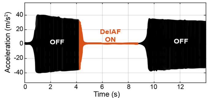
Fig. 8. Effect of the delayed acceleration feedback control on the chatter force of the HIL (Point A in Fig. 7).
