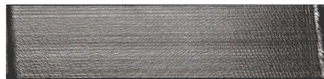
Fig. 18. Chatter marks on the milled surface for Workpiece II at N = 17000 rpm; parameters from Table 1 and 2.
