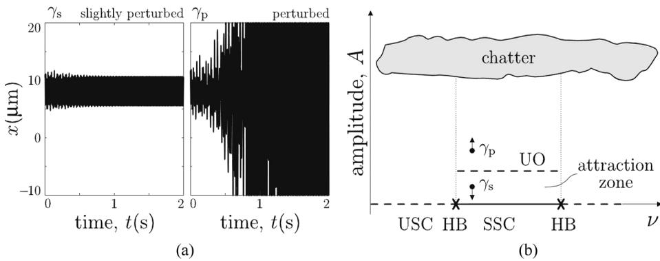
**FIGURE 6** (a) Time domain simulations at point  $\gamma$  with different perturbation levels. (b) Bifurcation structure along  $\nu$  (see Figure 3(b)). (HB: non-hyperbolic points related to Hopf bifurcation).
