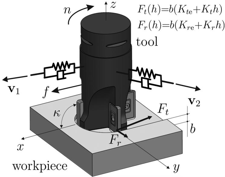
FIGURE 1 Schematic milling model.
