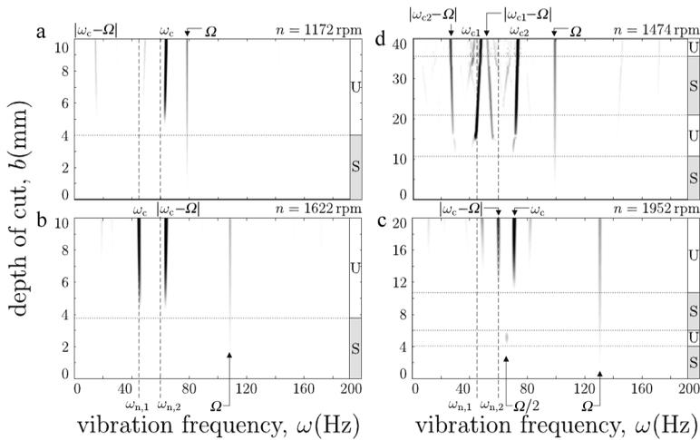
**FIGURE 5** Spectra of different time-domain simulations in different spindle speeds (see points A, B, C, and D in Figure 3).
