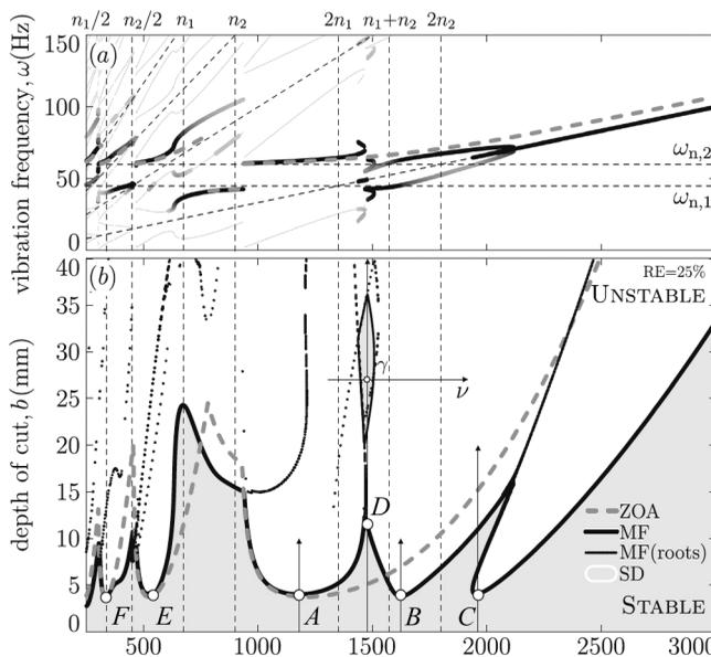
**FIGURE 3** (a) The frequency plot of the critically stable solutions using grayscale showing the strengths of the harmonics (Dombovari et al., 2011). (b) The linear stability of milling process (cf. Table 1).
