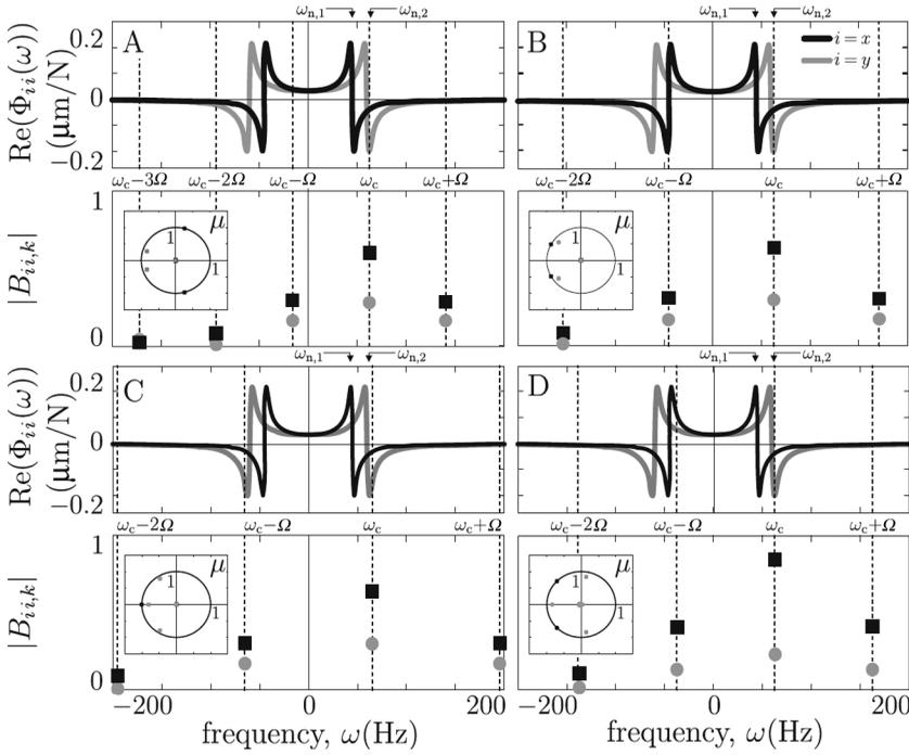
**FIGURE 4** The panels show the effect of the mode interactions (see Figure 3). In each panel the frequency response functions (upper panel), the harmonics of the directional factors, and the unit circles with the critical eigenvalues are presented.
