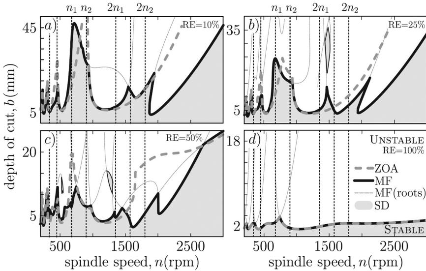
FIGURE 2 Stability charts in case of down milling processes with parameters taken from Table 1.
